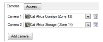
Adding a camera to an object will mean that, whenever there is an event on that object, the recording from that camera will be related to the time and date of the object event, in the Integration database.
